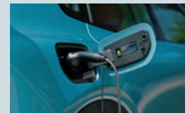
V2L SUPPLYING UP TO 6.6KW OF POWER TO EXTERNAL DEVICES
